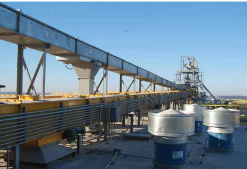
New 7,000-bph Zimmerman grain dryer served by 15,000-bph Intersystems wet and dry legs.
