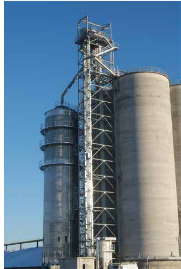
New 7,000-bph Zimmerman grain dryer served by 15,000-bph Intersystems wet and dry legs.
